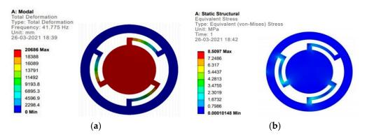
Figure 3. FEA of check-valves: (a) modal analysis; (b) static analysis.
